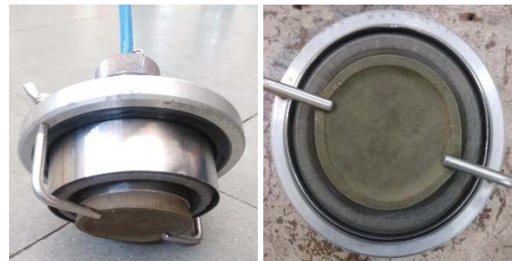
Figure 11: Regenerator flush with high pressure Nitrogen and petroleum Ether
