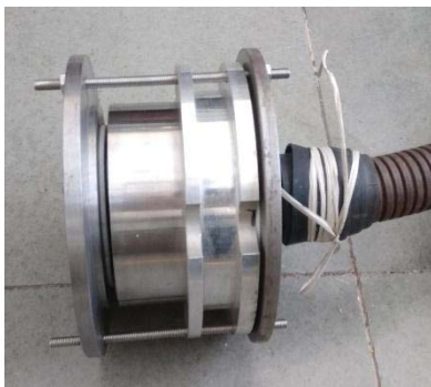
Figure 8: Regenerator flush with High pressure hot air blower
