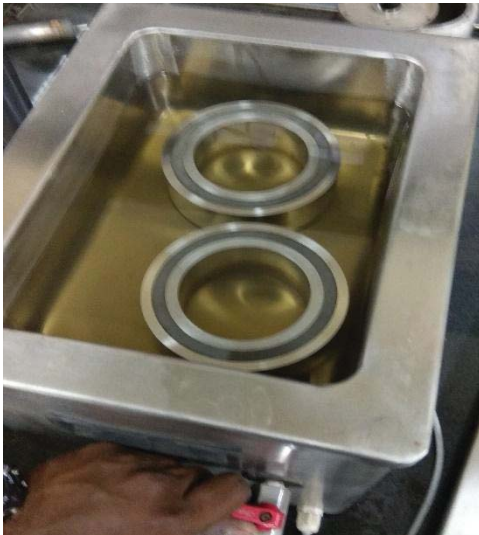
Figure 7: Regenerator Ultrasonic bath
