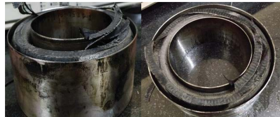
Figure 10: Loosened SS wire mesh
